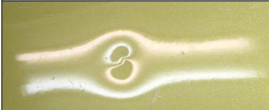
Example of small dent to be repaired on an Aluminum panel
