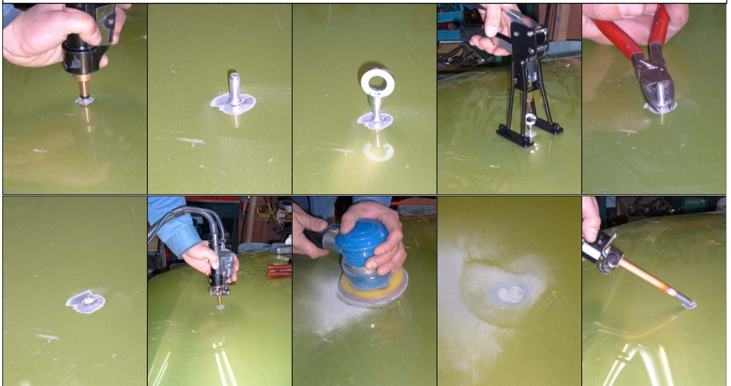
Example of the repair process to remove a dent from an Aluminum panel
